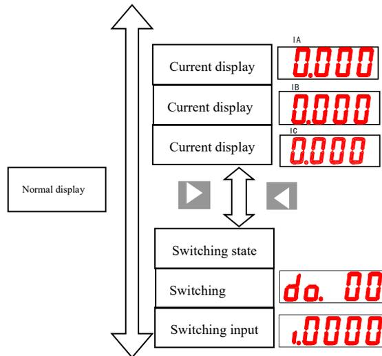
Note: Single-phase voltmeter is similar to AI menu structure, only one difference: voltage, frequency instead of current;
