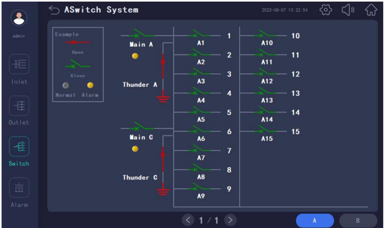
Determine how many incoming and outgoing lines there are based on the system drawings. It should be noted that if the system is not a one in one out or two in two out system, refer to the display pattern described in the parameter display section and switch status interface above.
