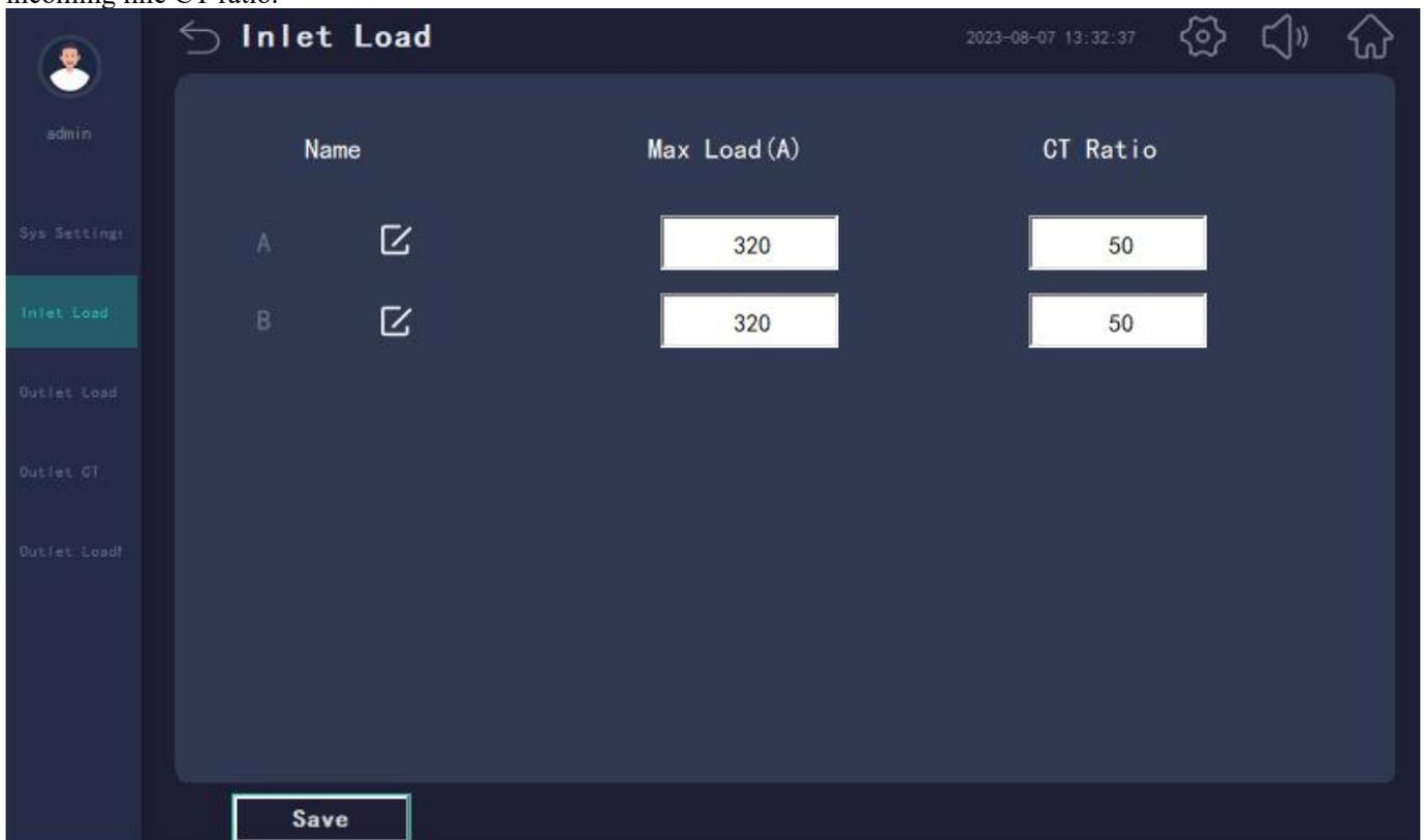
The load rating of the incoming switch is the indicated load current of the switch actually used. It is used to automatically calculate the overload limit value of incoming line load. Please refer to the alarm settings below to modify the load rating here. The default overload limit for the first section is 60% of the rated value here, and for the second section, it is 80%.
