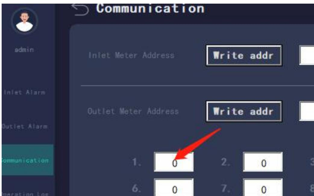
Write 10 in the input box to the right of the Write Address button in the slave address area, and then click Write Address. Click the read address button in the slave address area, and the box on the right displays 10, indicating successful modification. After modification, restore the address specified in the above regulations from the machine address settings.
