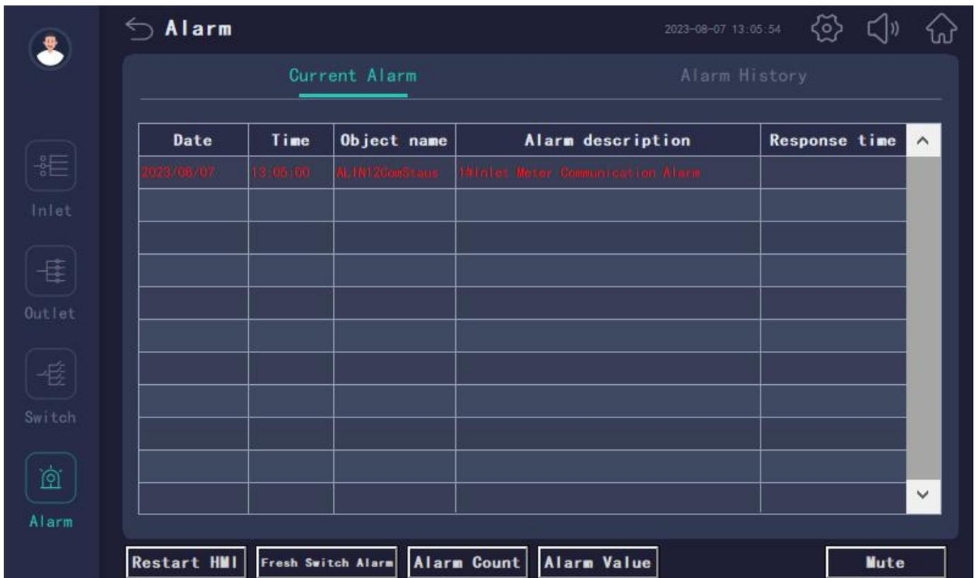
When an alarm occurs, the relay output of the buzzer and indicator light will act, and the screen will beep at the same time. The buzzer and buzzer relay output can be eliminated by clicking the Acknowledge Alarm button.
