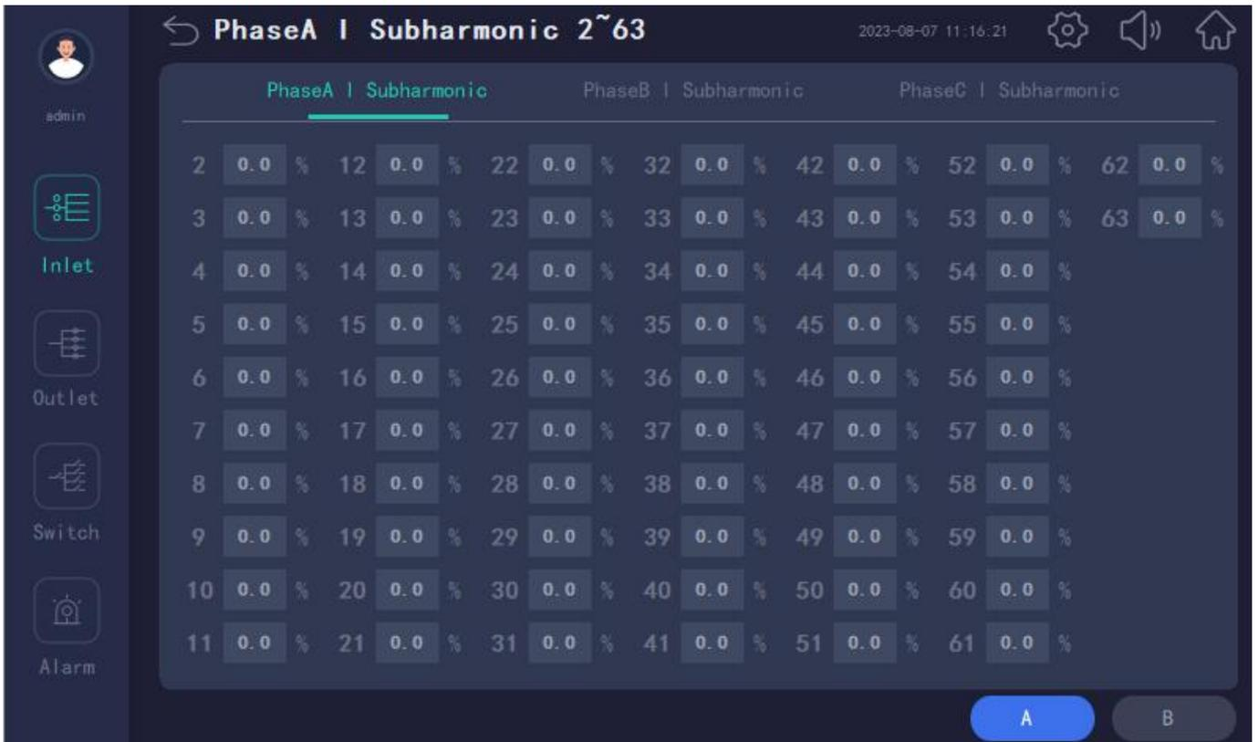
The third page is harmonic related parameters. You can view the fundamental active power, harmonic active power, fundamental active energy, and voltage total harmonics of each phase. Click the corresponding arrow to view the 2~63rd current subharmonic and voltage subharmonic of each phase.
