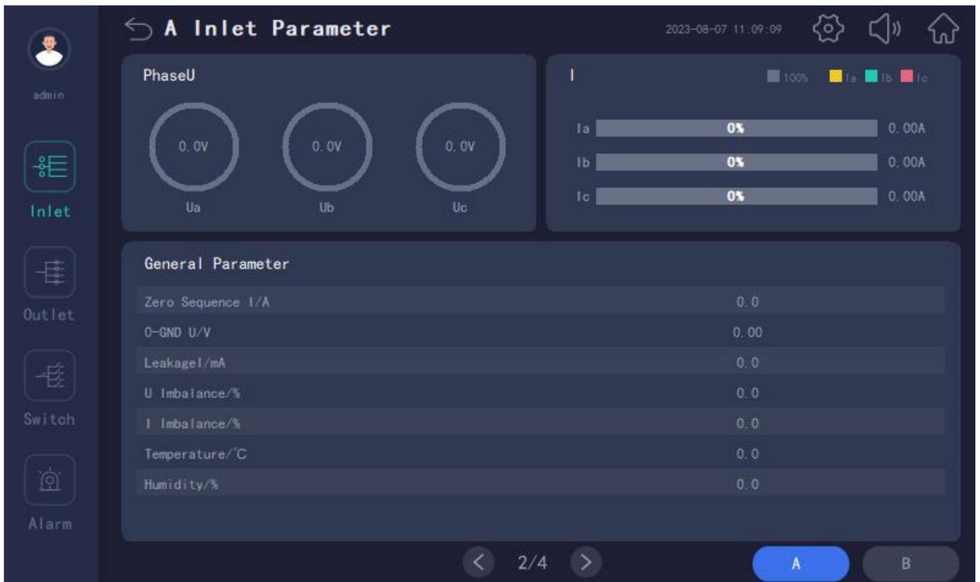
The parameters on page 2 include zero-sequence current, zero-ground voltage, leakage current, voltage unbalance, current unbalance, cabinet temperature, and cabinet humidity.
