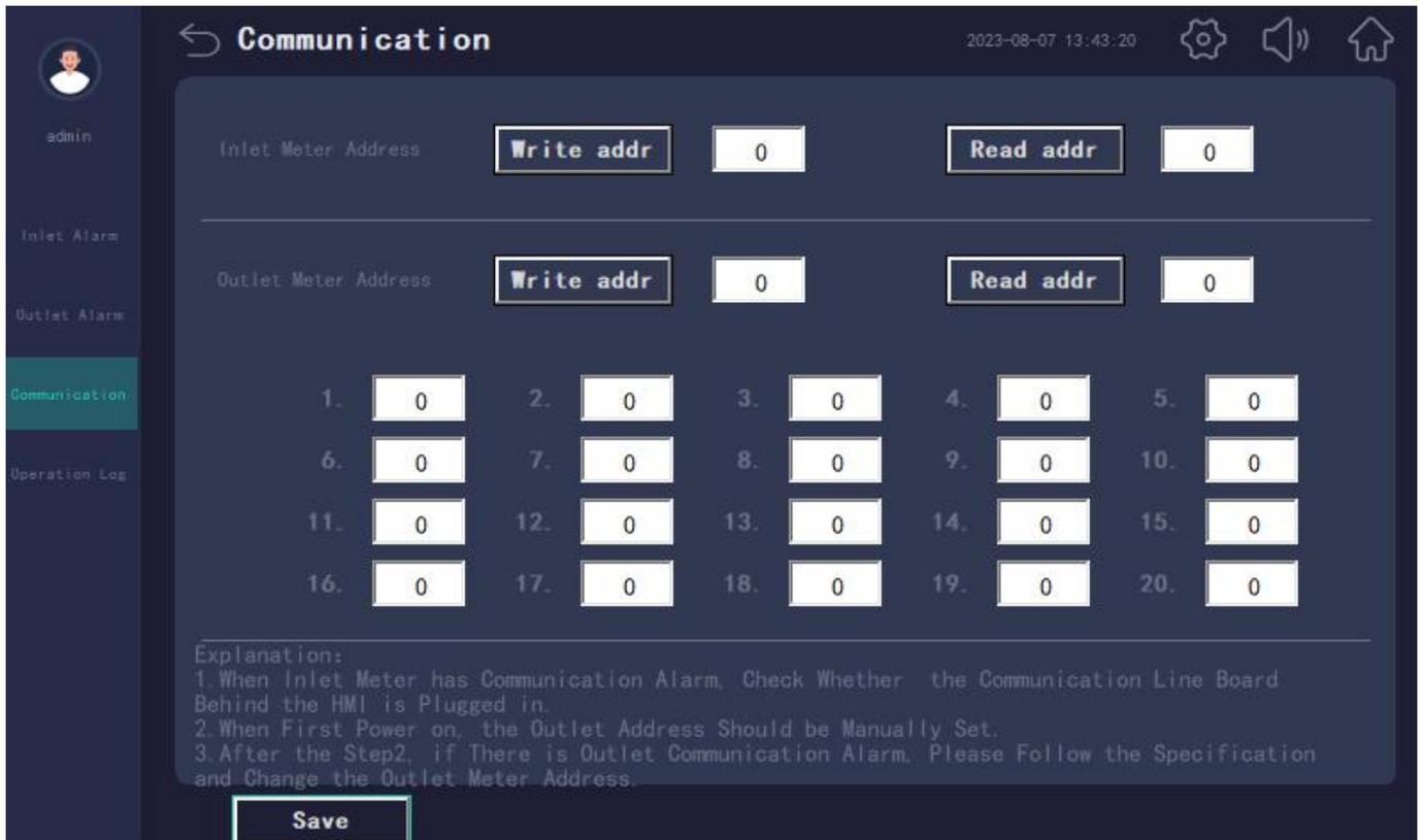
If the alarm message is "communication failure of incoming line module", check the address of the main module on this interface. The address of the main module should be 1. It is necessary to check whether the address of the main module actually used is 1. If it does not match, it needs to be changed to 1.
