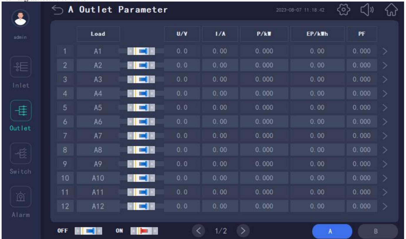
Outgoing parameters mainly include voltage, current, active power, active energy, and power factor.
