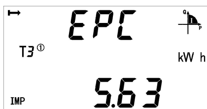
Current forward active energy on C phase
