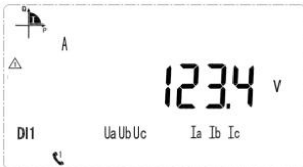
Voltage on A phase is 123.4V
