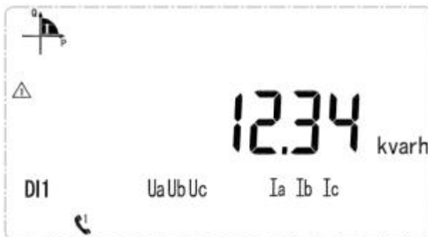
Current forward reactive energy 12.34kWh
