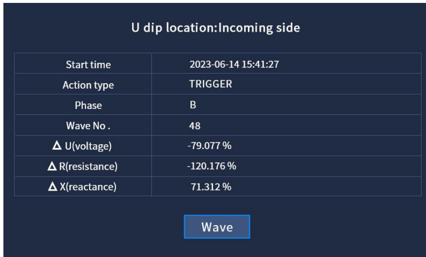
Fig. 4.25(a) Voltage dip location:incoming side
