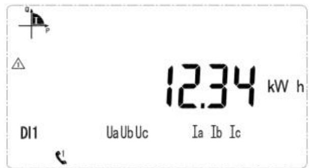
Current reversing active energy 12.34kWh
