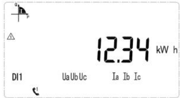
Current forward active spike energy 12.34kWh
