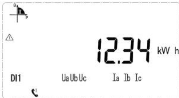
Current forward active energy 12.34kWh
